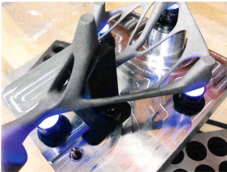
Hip tracker being adhesively bonded to Blue Photon grippers using UV light. This solution holds the part rigidly but without the distortion caused by clamping forces from plastic jaws.
