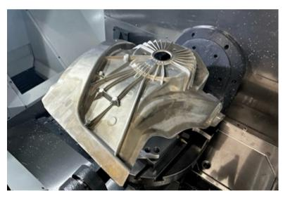
Soft material was not the EV strut housing's only workholding challenge: The part barely fit the UMC 750's travels. Potential fixtures needed to be low-profile enough to ensure the part continued to fit the machine. Images
