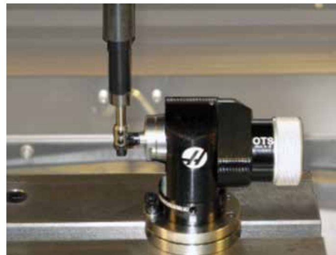
Figure 2. Use of a table mounted tool pre-setter to obtain gripper cleaning tool assembly length
