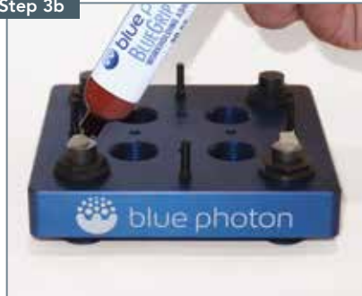
Apply enough adhesive to the grippers to fully fill the gap between the part and gripper.
