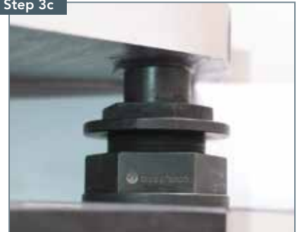
Position the part onto locators.
