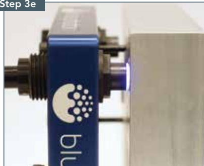
Polymerize the adhesive by applying UV light for 60 to 150 seconds.
