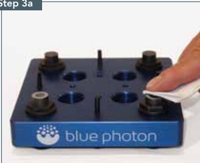
Clean dirt and oil from the grippers and workpiece.
