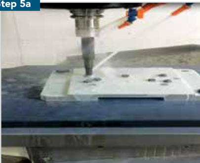
Loaded in CNC machine spindle (P/N 82400) to remove cured adhesive.
