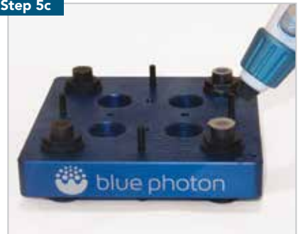
Remove residual adhesive with steam or hot water spray.
