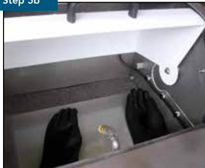
Spray the part and fixture with hot water.
