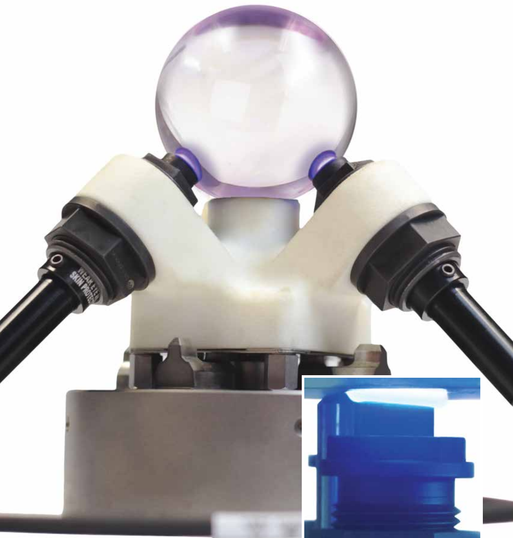
Gripper and insert components installed in an additive fixture. Adhering glass sphere with BlueGrip workholding adhesive.
