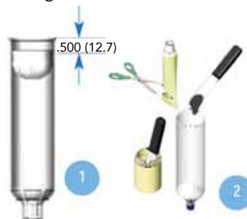
7. Place the filled cartridge reservoir into the retainer.
